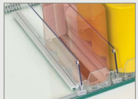
3 The lower fixing cams form a stable compartment when locking with the guide and stabilizer profile, specifically dividers (e.g. for round products on gravity shelves).
